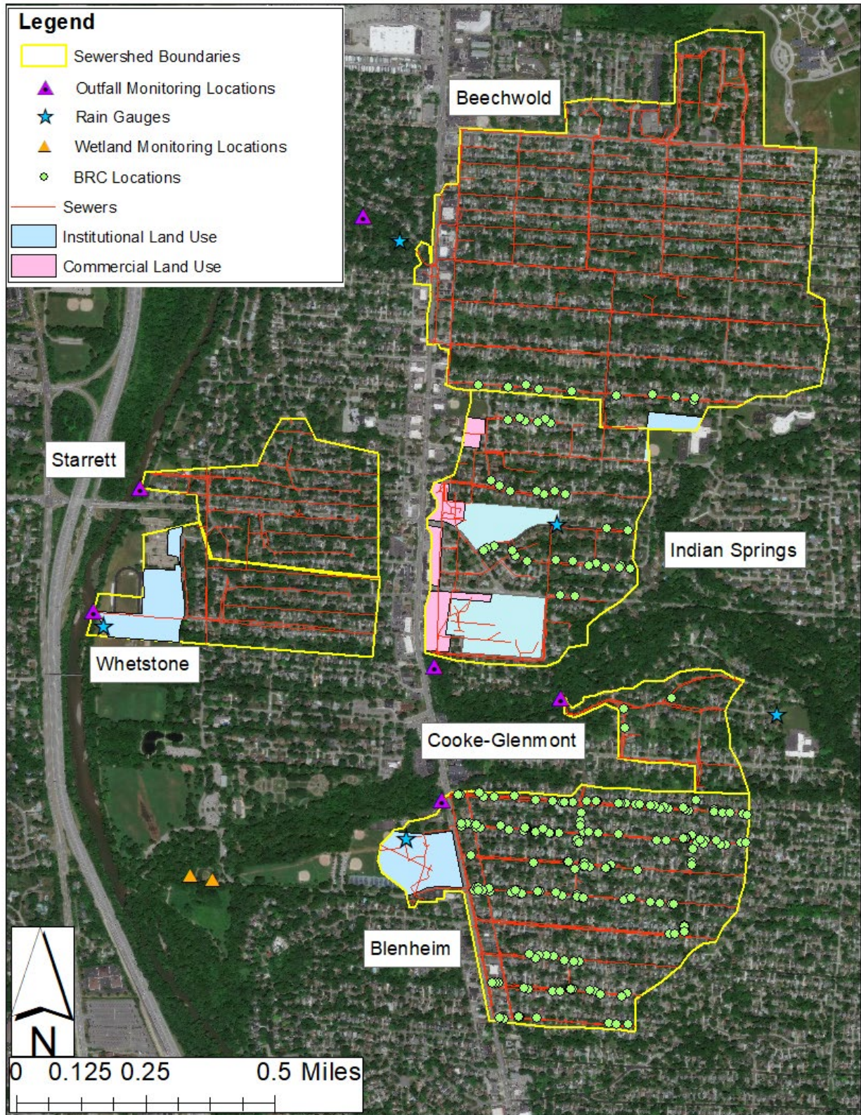
Figure 2: Boundaries of the six sewersheds monitored in this study. Distribution of bioretention cells (BRCs), monitoring locations, and land use within each sewershed are also shown. The remaining area within each sewershed not identified as commercial or institutional is residential.
