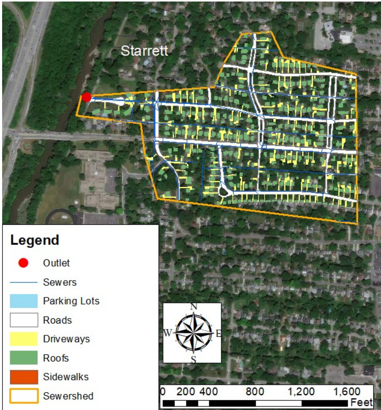
Figure 19: Map showing impervious surface types in the Starrett sewershed. Pervious areas in the sewershed are not highlighted with color.
