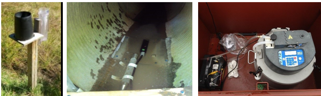
Figure 4: Rain gage cluster (left), sample intake (clear plastic) and area velocity meter (black) in the Cooke-Glenmont outfall (center), and automated sampler at Beechwold (right).
